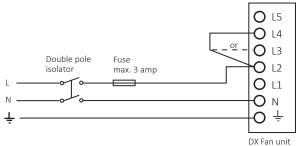
5.1.3 Basic Fan Operated By Remote Sensor
