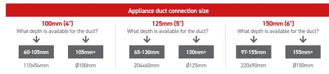
When a profile has been specified and the duct layout designed, the system resistance must be calculated to ensure that the appliance has sufficient power to more than match the resistance of the complete system.
