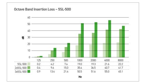
The diagrams illustrate the increased sound absorption levels when close-coupling up to three individual 0.5m lengths of rigid duct attenuators, thus reducing noise levels by up to 55dB.
