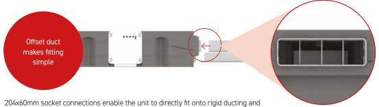
204x60mm socket connections enable the unit to directly fit onto rigid ducting and remove the need for additional adapters. For information on Domus rigid ducting, go to page 48. For Radial semi-rigid ducting, go to page 125.
