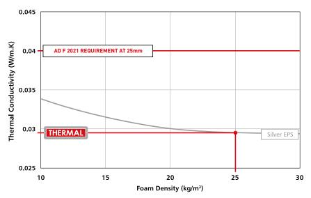
The Silver EPS used to manufacture Domus Thermal provides a significantly improved thermal conductivity value owing to the inclusion of carbon particles, which gives Domus Thermal its distinctive silver colour.
