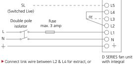
Connect link wire between L2 & L3 for supply
