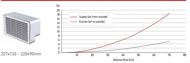
Performance data for double airbrick (code 905) with adapter (977)
